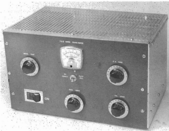
The transceiving converter is housed in a homemade aluminum cabinet which measures 8 \times 8 \times 12 inches. Perforated aluminum is used for the top and back sides of the cabinet to assure good ventilation.
