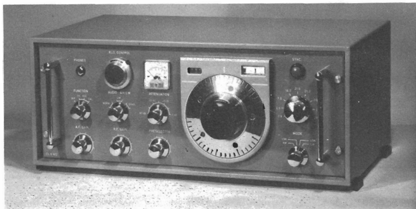
Front view of the receiver. At the upper left from the tuning-dial assembly is the receiver incremental-tuning control and the S meter, and at the upper right is the afc loop sync. push button. Within the dial assembly appear the dial counter in the window at the left, and the phase-lock meter indicator in the window at the right (an edge-wise meter is used). The home made dial was inspired by the design used in the HRO series of receivers.
