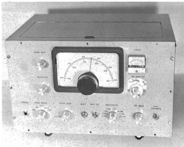
The W50MX receiver. Main tuning dial (J. W. Miller, MD-7) has both 6:1 and 36:1 tuning ratios. A 6:1 planetary drive assembly (Arrow Electronics, Type 4511) is used on the preselector tuning capacitor. The pointer is homemade. (Photos by A/3C Michael M. Steinbacher)
